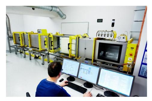
The test rig for testing and classifying coarse dust and fine dust filters can now also be used for particulate filters.
