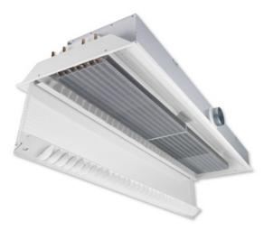
DID642 active chilled beams come in sizes from 900 to 3000x600x170 mm (LxHxD) and have been designed for a cooling capacity of up to 2600 W or a heating capacity of up to 3500 W, and for volume flow rates of 8 to 85 l/s or 30 to 300 m<sup>3</sup>/h.
