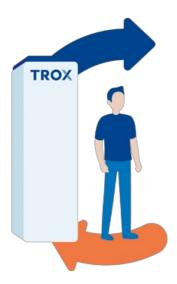
The TROX AIR PURIFER vents cleaned air into a room above head height. This allows the unit to disperse a high-volume air output without creating draughts. At the same time, it also prevents viruses from an infected person from spreading directly via the
