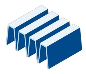
In contrast to conventional flat filter plates, the filter panels in the TROX AIR PURIFIER are concertinaed. As a result, the unit has a total filter area of 47  $\rm m^2.$
