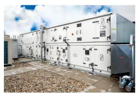
Thanks to their modular design, TROX X-CUBE air handling units can be perfectly adapted to fit any conditions. They can be individually configured and are hence suitable for a wide spectrum of applications. More than 70 sizes are available, and they are designed for volume flow rates of 600 to  $100,000 \, \text{m}^3\text{/h}$  at an airflow velocity of 2 m/s. X-CUBE units are available as supply or extract air units or as a combination of both.
