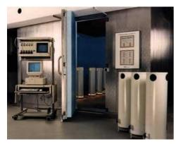
This facility is used for the standardised identification of the cooling capacity of passive water cooling systems according to standards DIN EN 14240, 14518 and 15116. This is where new developments are advanced, catalogue data determined and measurements are taken as proof of performance for major projects according to customer wishes.
