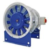
X-FANS smoke exhaust fans remove the smoke gases from the individual fire compartments in the garage. Customers have a choice of different constructions for various temperature ranges, depending on the garage layout.
