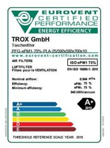
If, for example, you compare an air filter of category ePM1 > 50% (formerly F7) of class A+ having a energy consumption of maximum 800 kWh with a filter of class D having a energy consumption of maximum 2000 kWh, at an energy price of (just) 15 cent/kWh the energy costs are  $\leq$ 120 per year for energy efficiency class A+ compared to  $\leq$ 300 for class D. The difference amounts to  $\leq$ 180 for a single filter element.
