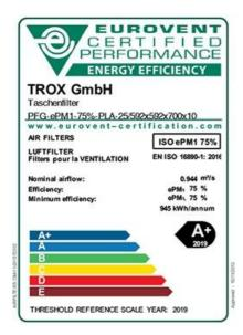
If, for example, you compare an air filter of category ePM1 > 50% (formerly F7) of class A+ having a energy consumption of maximum 800 kWh with a filter of class D having a energy consumption of maximum 2000 kWh, at an energy price of (just) 15 cent/kWh the energy costs are  $\[ \in \]$ 120 per year for energy efficiency class A+ compared to  $\[ \in \]$ 300 for class D. The difference amounts to  $\[ \in \]$ 180 for a single filter element.
