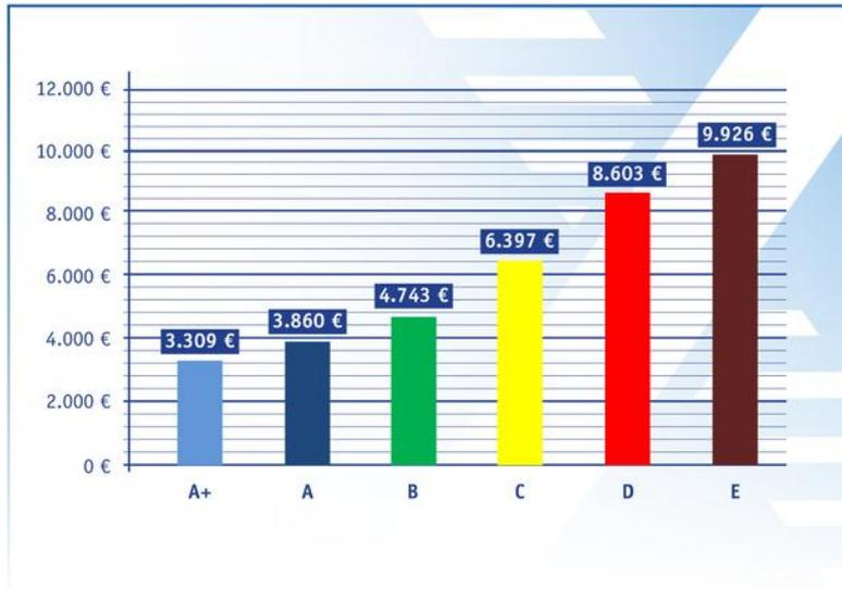
*Within the period of one year, one pocket filter of filter class F7 according to EN779, using a volume flow rate of 100,000 m<sup>3</sup>/h, consumes EUR 8603.00 in energy efficiency class D and EUR 3309.00 in energy efficiency class A+. Changing the filters from energy efficiency class D to A+ results in an annual energy costs saving of 61% (EUR 5294.00).*
