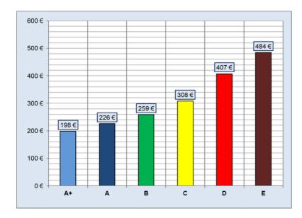
Within a period of one year, one pocket filter of filter class ePM1 75% according to ISO16890, using a volume flow rate of 3.400 m3/h consumes EUR 407 in engery efficiency class D and EUR 198 in engery efficiency class A+. Changing the filters from energy efficiency class D to A+ resukts in an energy costs saving of 51% (EUR 209).
