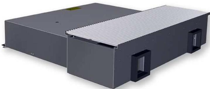
*The FSL-U-ZAS under floor unit has a maximum height (including grille) of only 195 mm (maximum height when installed in a false floor: 140 mm) and a maximum length of 1150 mm; it is hence ideal for refitting ventilation and air conditioning systems in refurbishment projects.*
