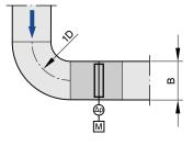
A bend without additional straight upstream flow length in front of the VAV control unit has no significant influence on the volume flow rate accuracy  $\Delta q_v$ .
