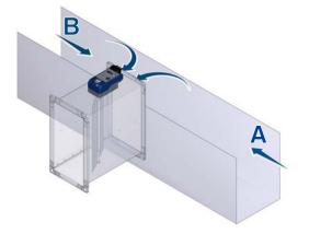
For airflow direction A in the main duct: specified volume flow rate accuracy  $\Delta q_v$  achievable.
