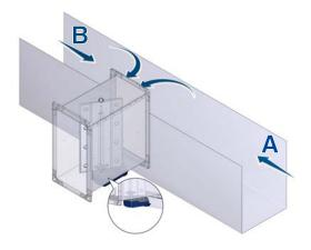
For airflow direction A in the main duct: for the specified volume flow rate accuracy  $\Delta q_{_{\nu}}$  a surcharge of 10 % must be taken into account in the upper third of the nominal volume flow range.
