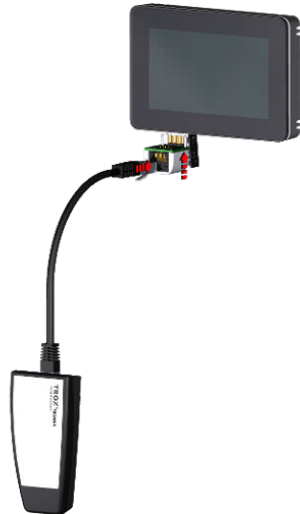
Fig. 8: Connection with configuration adapter and BlueCON Bluetooth adapter
