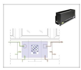
The ready-to-use, decentralised SCHOOLAIR-B and FSL-B units create an inducing displacement flow and use pumped hot water and pumped chilled water for heating and cooling.
