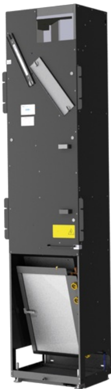
Vertical supply air and extract air unit FSL-V-ZAB with heat exchanger and heat recovery bis 42 l/s bis 150 m 3 /h B: 396 mm H: 1.800 mm T: 319 mm
