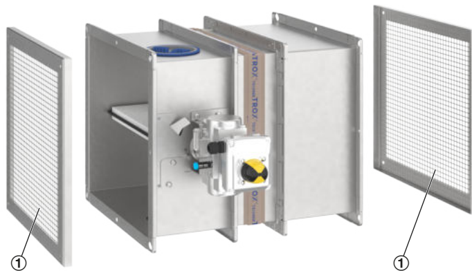
① Cover grille, mesh aperture 10 mm × 10 mm, wire width 2 mm
