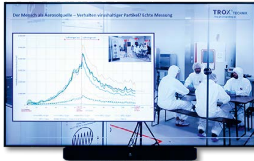
Measurements in the laboratory, which was occupied by four people, showed that the viral load can be significantly reduced with an air purifier.
