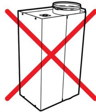
Fig. 14: Installation orientations for TVR-Ex with pneumatic control
