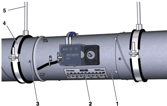
Fig. 11: Installation example using a VAV terminal unit TVR-*
