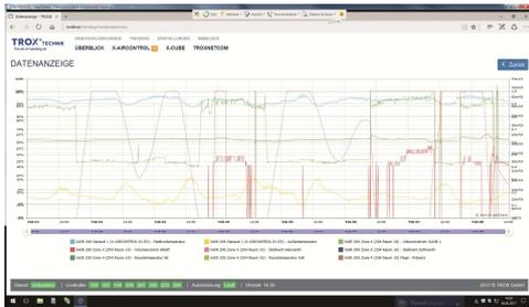
*X-TAIRMINAL allows users to display and analyse all parameters for a ventilation and air conditioning system, for example to recognise trends.*
