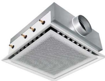
*DID614 active chilled beams are available in two sizes, 600 x 600 mm square or 1200 x 600 mm rectangular; they are designed for a cooling capacity of up to 2 000 W or a heating capacity of up to 1600 W and for volume flow rates from 8 to 70 l/s or 30 to 250 m<sup>3</sup>/h.*
